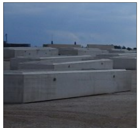
8000mm x 2100mm x 1.205m precast concrete box sections ready for shipment to the job site
