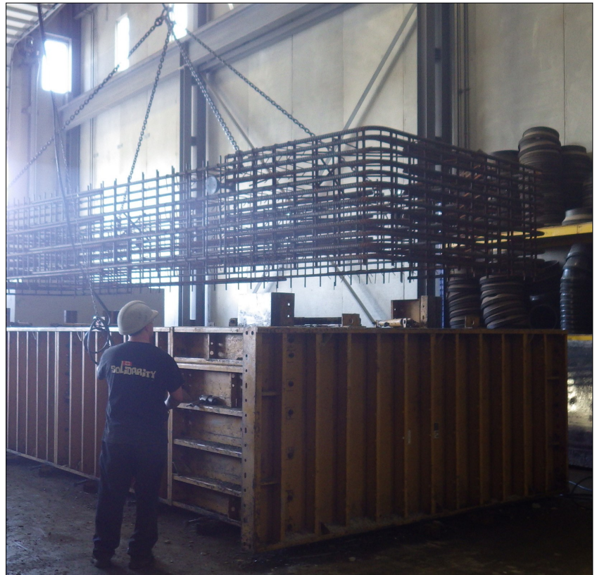
Pre-welded cage being lowered into the mold jacket
