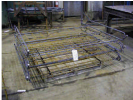
Pre-welded step assembly ready for shipment and immediate use.
