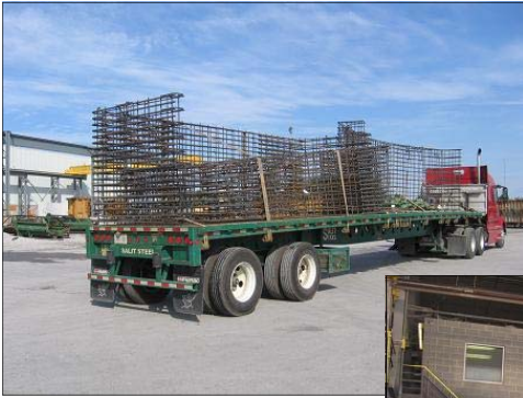
Pre-assembled reinforcing cages arrive at the precast plant on a predetermined schedule. The assemblies are offloaded in the plant, directly from the flatbed to the mold.
