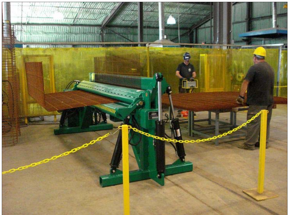
Double bender purchased from Elk River Machine Company now operational at StelCrete's Welland facility to increase efficiency in fabricating mesh assemblies. A U-shaped cage segment can be bent without removing the steel mat from the bending table. The ERMC double bender includes an unobstructed bending deck.
