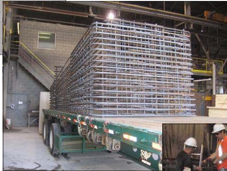
Pre-assembled reinforcing cages arrive at the precast plant on a predetermined schedule. The assemblies are offloaded in the plant, directly from the flatbed to the mold.
