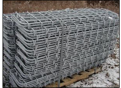
Pallet of galvanized pre-welded reinforcing mats ready for shipment to Central Precast.
